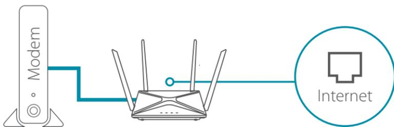
**Note:** If your router does not have a port labeled as INTERNET, plug the Ethernet cable into LAN Port 1.
